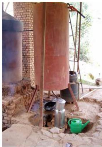
**Figure 2: Distillation of Organic Geranium Oil at Ikerezi**
