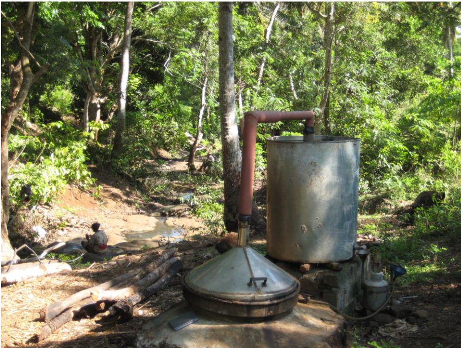
Field still for distillation of ylang ylang, Comoros Islands
