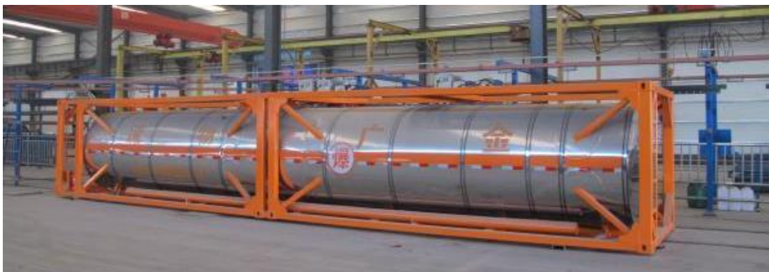
Figure 8 - an example of a 20ft .ISO palm oil tank container
